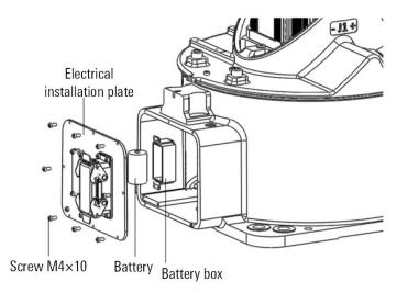
Figure 12-5 Remove manipulator electrical installation panel
