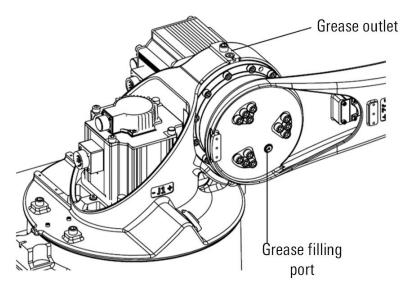
Figure 12-7 Replace the grease of J2 axis reducer
