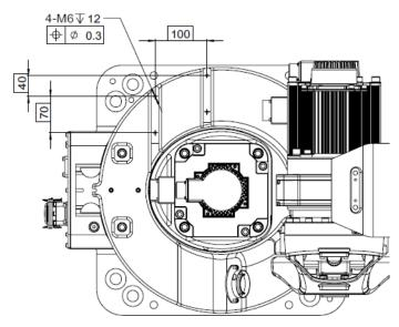
Figure 7-8 Diagram of shoulder interface
