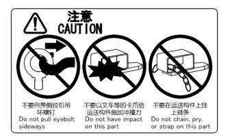
Figure 9-1 Precautions for manipulator during handing
