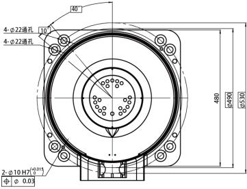
Figure 4-1 Dimensions of the manipulator base interface
