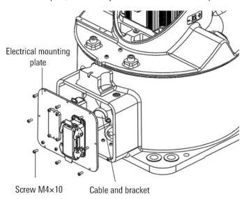
Figure 12-2 Base internal cable
