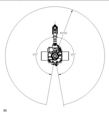
Figure 7-1 Working range of AIR25-1700B manipulator
