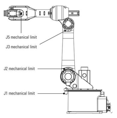
Figure 7-2 Mechanical brake on the manipulator
