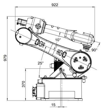
Figure 9-3 Handling posture of AIR25-1700B Manipulator
