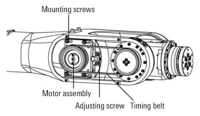
Figure 12-10 Removal of synchronous belt
