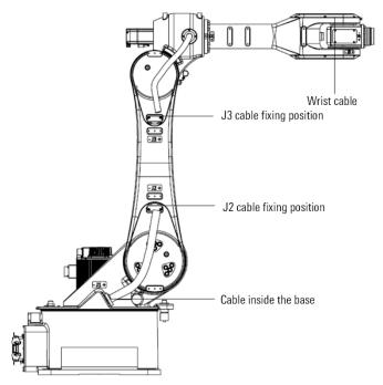
Figure 12-1 Layout for cables of manipulator
