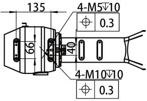
Figure 7-6 Diagram of elbow load of the manipulator
