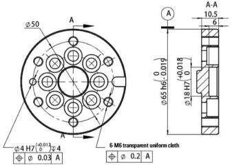
Figure 7-3 The flange dimension diagram of wrist
