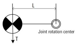
Figure 7-4 Diagram of load eccentricity
