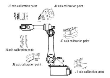
Figure 8-1 AIR25-1700B zero point diagram of each axis
