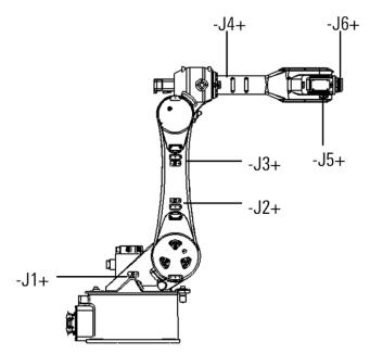
Figure 2-3 Direction Sign of each joint on manipulator
