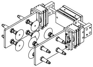
Figure 6-2 Suction cups for industrial robots
