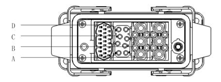
Figure 5-1 The heavy-duty connector on AIR25-1700B manipulator body
