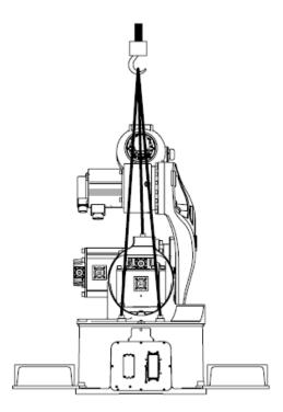
Figure 9-5 Diagram of AIR25-1700B Manipulator handling with swinging ring
