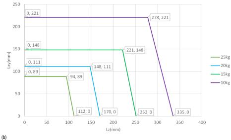
Figure 7-5 Location of wrist load center of AIR25-1700B manipulator
