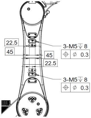
Figure 7-9 Diagram of upper arm interface
