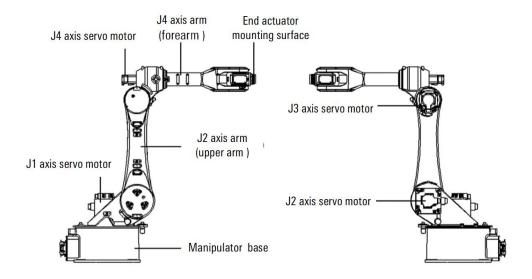
Figure 1-2 AIR25-1700B Robot Body and Its Various parts
