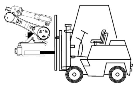
Figure 9-4 Diagram of AIR25-1700B handling with forklift
