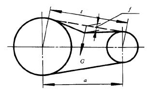
Figure 12-11 Installation deflection of synchronous belt
