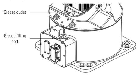
Figure 12-6 Replace the lubricating grease of J1 axis reducer
