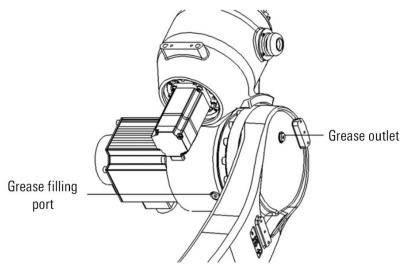
Figure 12-8 Replace the lubricating grease of J3 axis reducer
