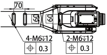
Figure 7-7 Diagram of the manipulator forearm
