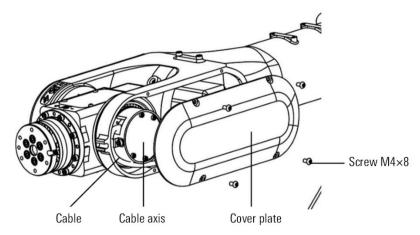
Figure 12-4 Inner cable of the wrist
