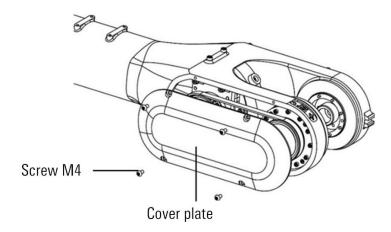
Figure 12-9 Removal of cover plate
