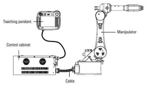
Figure 1-1 Composition of Robot System
